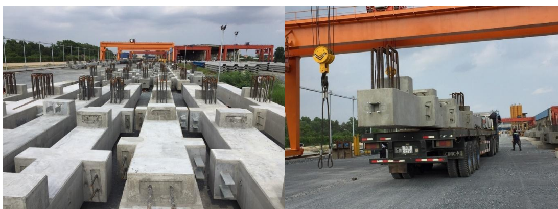
Figure 1. 8 Pipe Rack Column - the largest prefabricated precast concrete component in Viet Nam at Phan Vu Infrastructure Construction Co., Ltd
