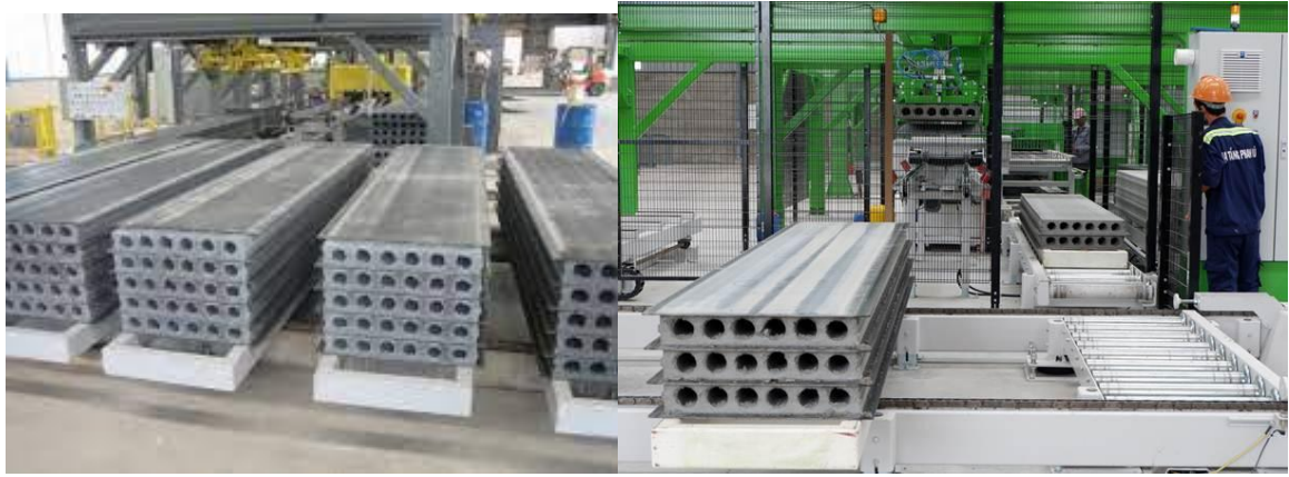
Figure 1. 10 Acotec and Eurowall hollow wall panels at Xuan Mai Concrete Factory (Hanoi)
