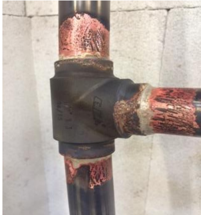
© Dennis Huehren Copper to brass joint (uncleaned)
