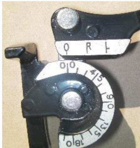
Figure 34: Angle marks on a tube bender (Source: HEAT GmbH)
