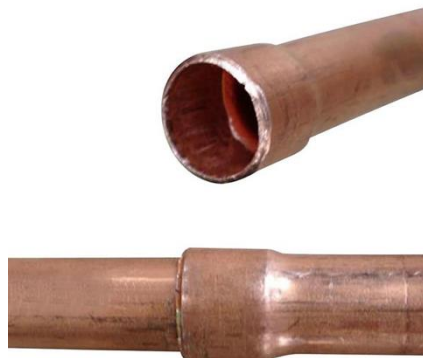
Figure 2-26: Swaged joint (Source: HEAT GmbH)
