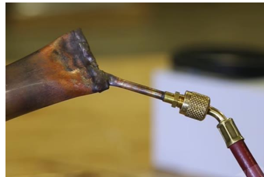
Figure 4-3: Schrader valve at a squeezed copper tube for OFDN supply (Source: HEAT GmbH)
