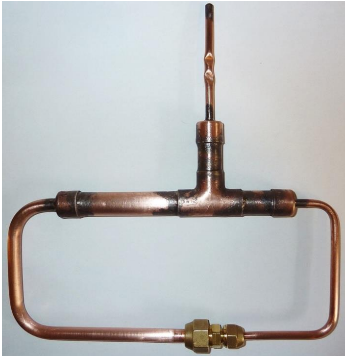
Figure 5-2: Practical brazers' examination specimen example (including bending and flaring) (Source: HEAT GmbH)
