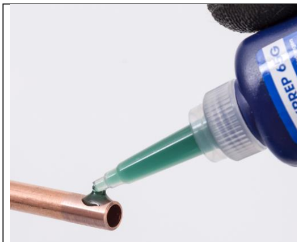
Figure 6-27: Applying LOKPREP to a pipe end (Source: Vulkan)
