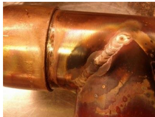
Figure 1-12: Example of welded copper tube joint (Source: HEAT GmbH)
