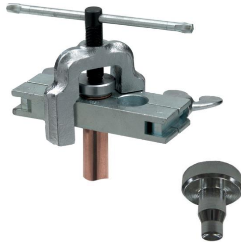
Figure 2-25: Swaging bar and die (Source: ITE)
