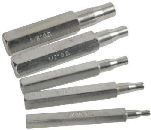
Figure 2-24: Swaging punches for the use with hammer (Source: ITE)
