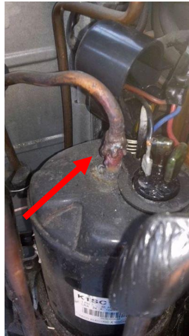
Figure 4-20: Example of bad brazing joint (Source: HEAT GmbH)
