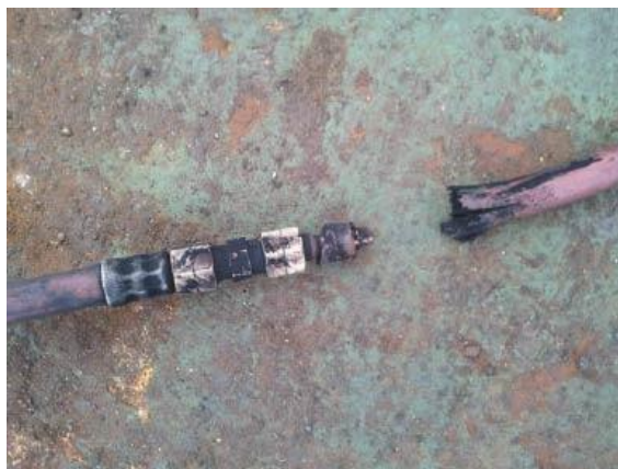
Figure 3-11: Hose burn from flashback in oxygen and acetylene hose (Source: EIGA)
