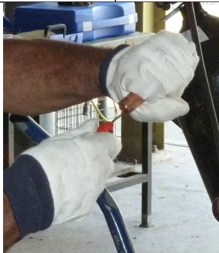
Figure 4-7: Deburring with pen-styled deburrer (Source: HEAT GmbH)
