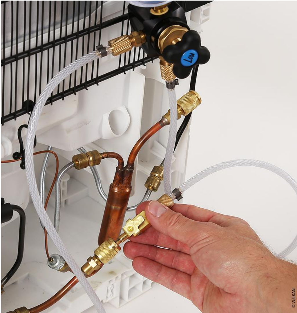
Figure 6-33. Exemplary refrigerant circuit servicing arrangement (Source: Vulkan)
