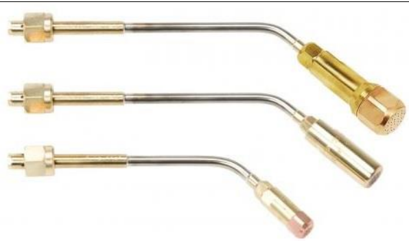
Figure 3-5: Brazing (shower) nozzle attachment for larger copper tube diameters and high energy flow; acetylene or propane (Source: www.Perkeo)
