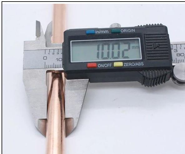
Figure 6-26: Example of the use of a calliper gauge (Source: HEAT GmbH)
